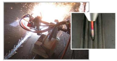
The Arcair-Matic® N7500 gouging system is highly productive for any metal fabrication operation where gouging and welding represents a large portion of the work schedule. This applies to almost all metals, including stainless steel, carbon, manganese, and chrome-moly steels.
